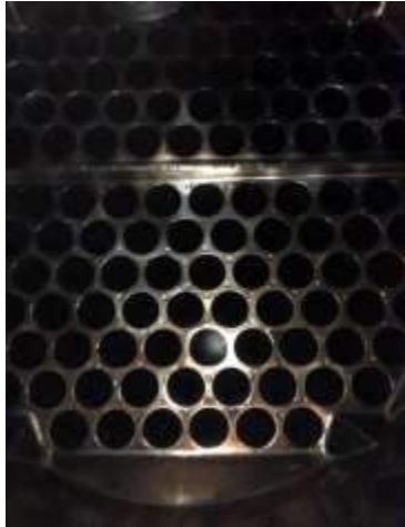
Top of skim milk evaporator tube chest
